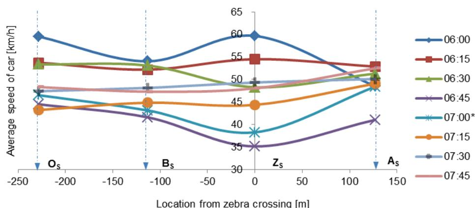
Figure 5 Average speeds (km/hr) of car on Sukowati West Street [Mantingan – Solo, 06:00 – 08:00]
